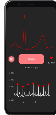
On-device ECG identity verification: live R-peak detection and accept/deny.
